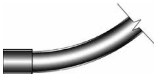
Standard PVC Coupling bonded onto fiberglass elbow.
